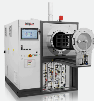
GLO 120/11-1G automatic up to 1100°C with optional hydrogen package and drawer door
