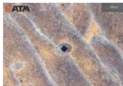
Fig. 4: Hardness: 129 HV0.1, tested in the center of the cross-section - 10x
