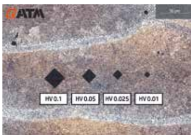
Fig. 3: Comparison of Vickers indentation sizes - 20x
