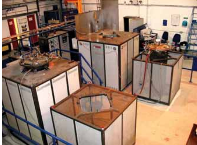
Two similar installations of bespoke toploding furnaces for surface treatment of turbine blades. Once lifted from the furnaces the controlled atmosphere retorts are placed into a cooling station.
