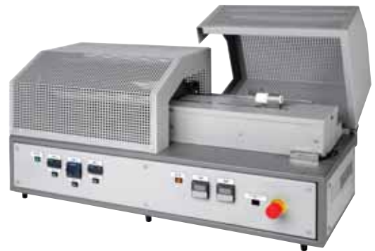
A bespoke thermal cycling system for extended testing of temperature sensors between ambient and 1200°C over thousands of repetitions
