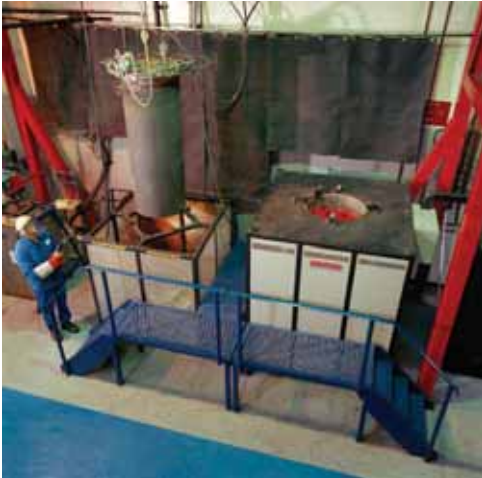
Two similar installations of bespoke toploding furnaces for surface treatment of turbine blades. Once lifted from the furnaces the controlled atmosphere retorts are placed into a cooling station.
