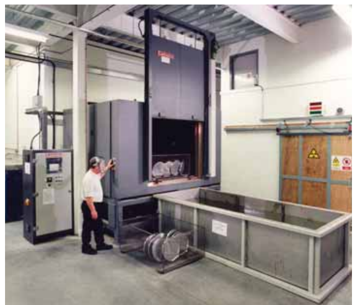
A bespoke LGP 600°C 2600 litre oven with load management system & quench, conforming to the requirements of AMS 2750D for Class 2 Thermal Processing Equipment with Type D instrumentation.
