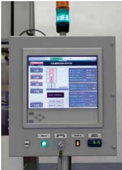
Bespoke thermal test rigs. One for evaluation & calibration of thermal indicator paints that are used in aerospace turbine blade manufacture. The other for extended cycling from ambient temperature to 1200°C to test turbine blade barrier coatings
