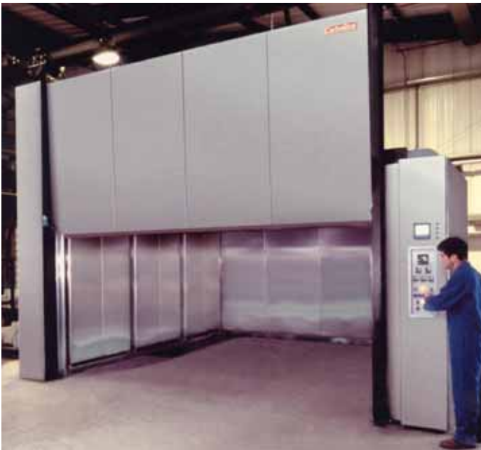
A bespoke LGP large general purpose 300°C oven used for drying aerospace components
