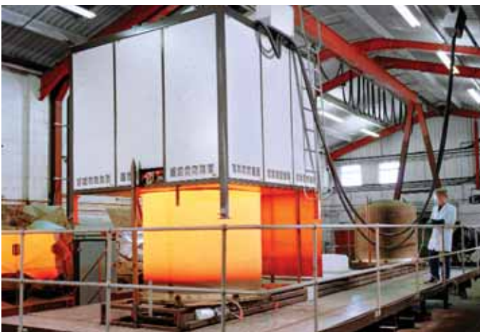
A bespoke 1100°C top hat furnace system for a proprietary turbine blade coating technique. Comprising of 2 working hearths, 2 retorts an atmosphere control system & a furnace chamber.
