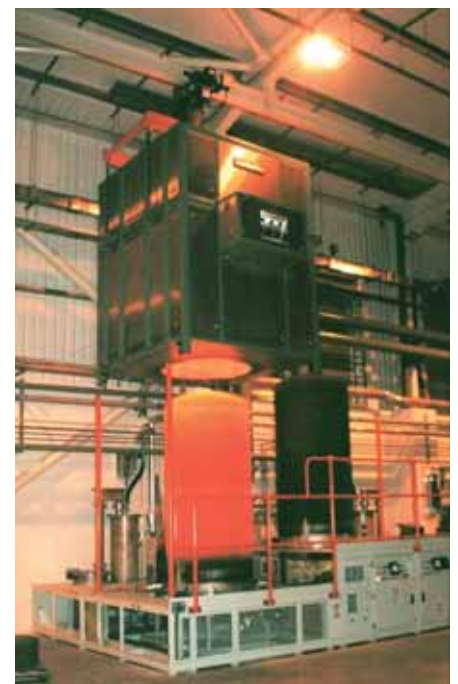
A bespoke top hat system for pack aluminising turbojet turbine blades at temperatures up to 1150°C under a controlled atmosphere
